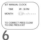
Press two Number buttons for the month, two Number buttons for the day, and two Number buttons for the year. For example, for July 1, 2000, press 07, 01, 00. The day of the week will appear automatically.
